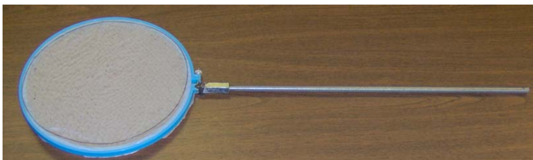
Figure 82 - Sail Frame with Attached Metal Rod
