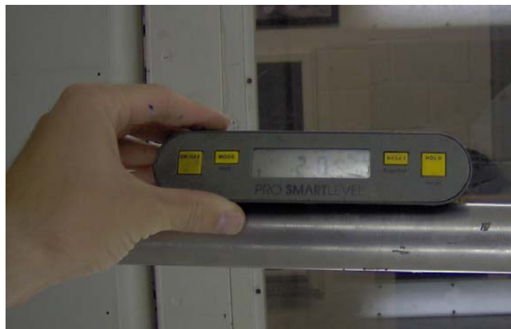
Figure 10 - Pitch Angle Adjustment in the Wind Tunnel
