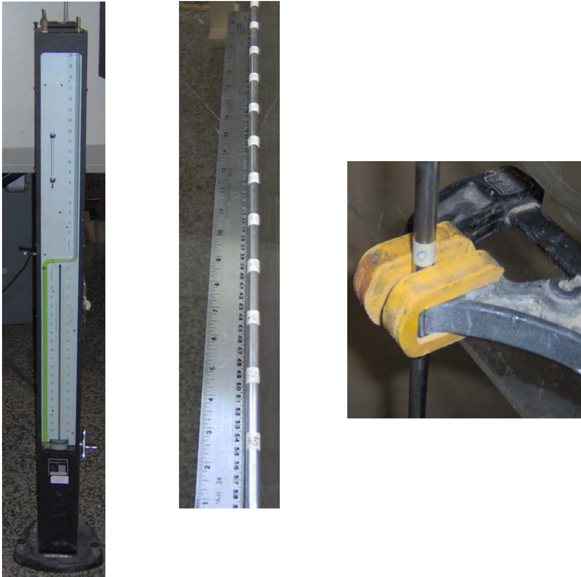
Figure 98 - Pitot-Static-Tube Read-Out Device (left), Marks (center) and Mounting (right)
