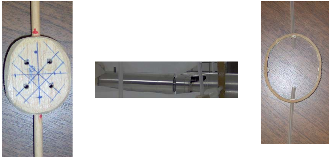
Figure 29 - Center Piece, Balance Sleeve and Rod Bypass
