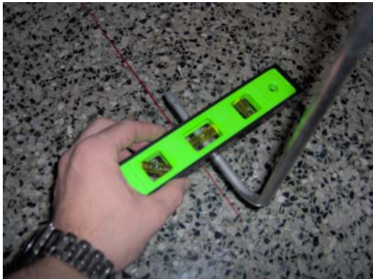
Figure 99 - Adjustment of the Pitot-Static Tube Pitch Angle (left) and Yaw Angle (right)
