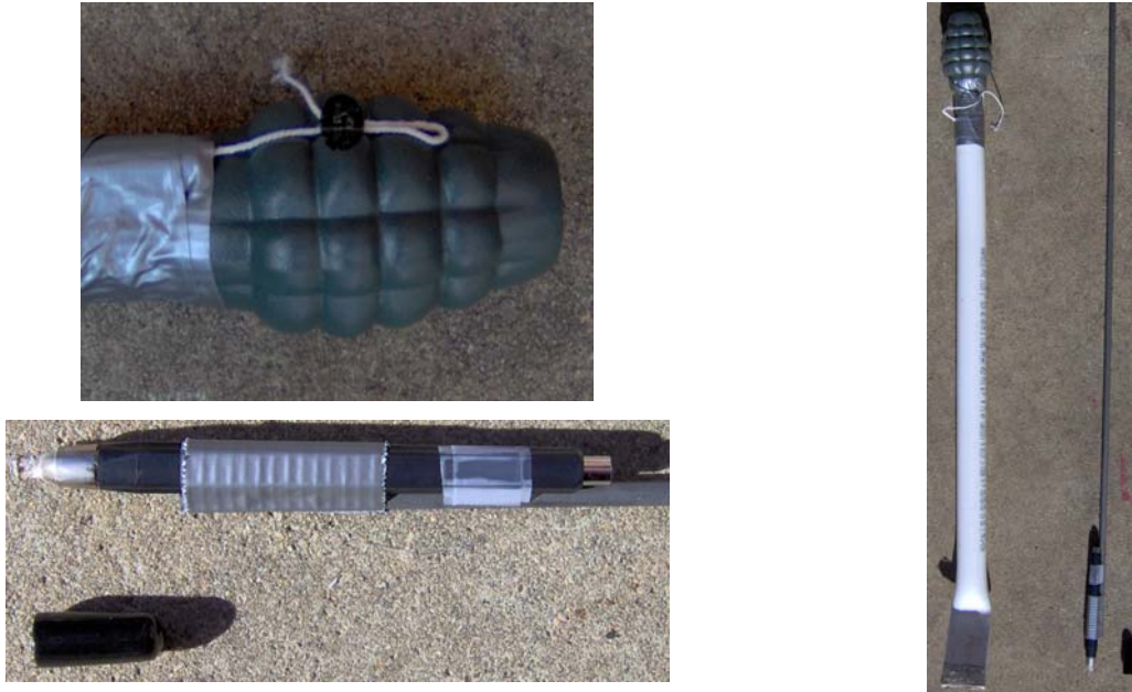
Figure 104 - Smoke Grenade, Smoke Pen (left) and Smoke Duct, Smoke-Pen on a Stick (right)
