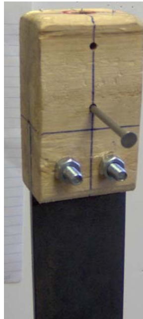
Figure 31 - Yaw Fixing Device in the Wooden Sleeve
