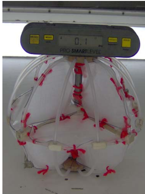
Figure 47 - Initial Pitch Angle Determination and Adjustment of the tTED2
