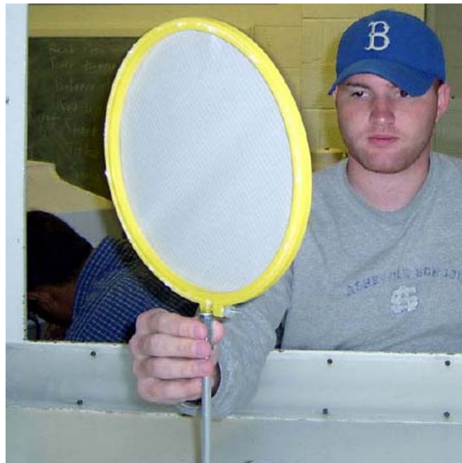
Figure 81 - Sail Frame Placed in the Wind Tunnel from [25]
