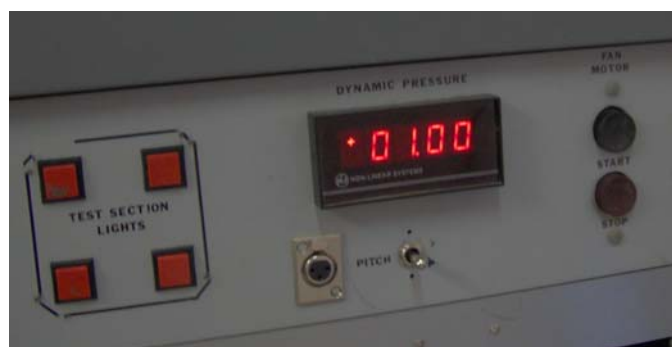
Figure 8 - Wind Tunnel Main Control Panel
