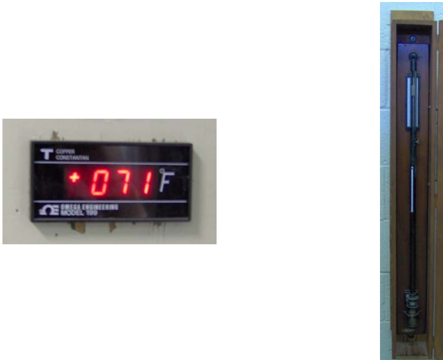
Figure 9 - Thermometer (left) and Barometer (right) in the Wind Tunnel Room
