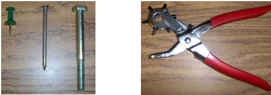
Figure 83 - Tools Used for Punching in the Holes
