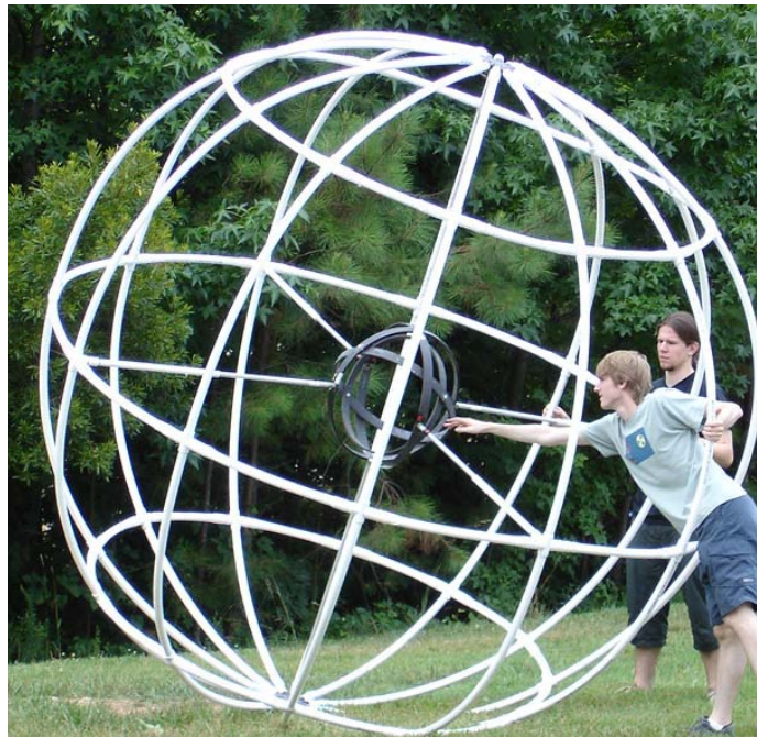
Figure 18 - Gimbal Supported to the Outer Structure
