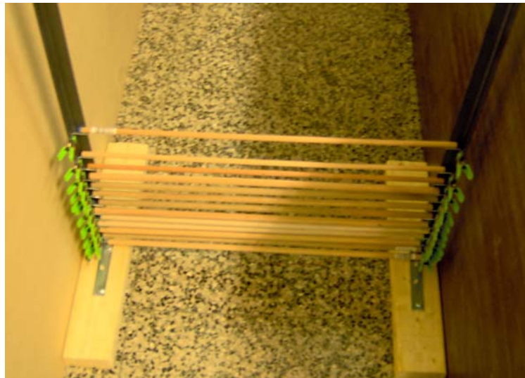
Figure 97 - Shear Grid in the Improved Smoke Channel
