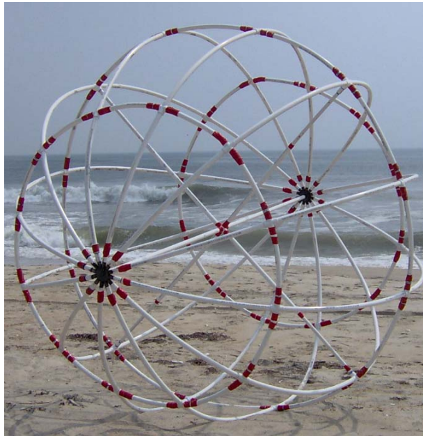
Figure 19 - TED Outer Structure, 6-way Center Piece and Inner Struts
